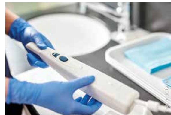
The handheld imaging device combines an intraoral camera and an applicator.
